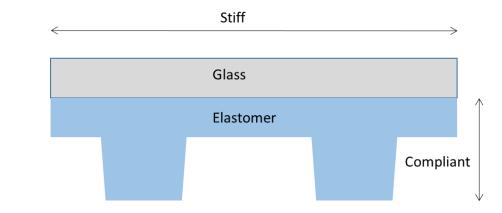
Low-pressure injection molded silicone rubber on glass backing, with lithographically-defined "posts" for selective transfer.
