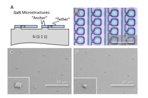
microLEDs suitable for micro assembly with elastomer stamp:
