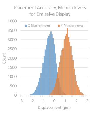
displacement at 3o: +/- 1.5 µm
